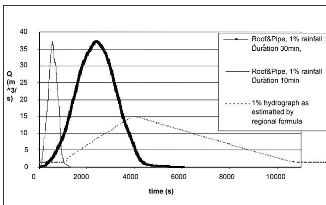
Figure 5 : comparison of 3 possible 1% probability hydrographs at abscissa 1501 : with Roof&Pipe for durations 30 and 10 min, with regional formula
