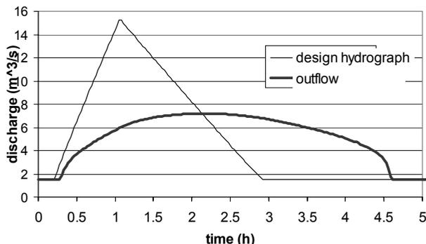
Figure 4 : mitigation of flood through the proposed dry reservoir, 1% probability hydrograph, 1m x 1m sluice (RubarBe computations)
