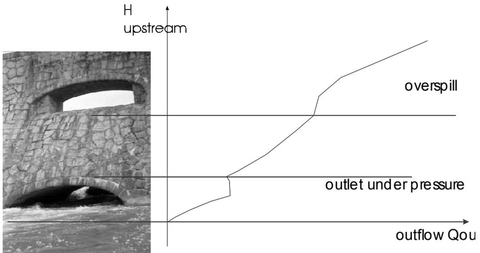
Figure 3: Example of rating curves water height/outflow used for simple hydraulic computations with regard to the different stages
