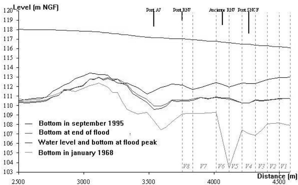
Figure 4 Calibration of the model on the 1000 year flood (Balayn, 2001)
