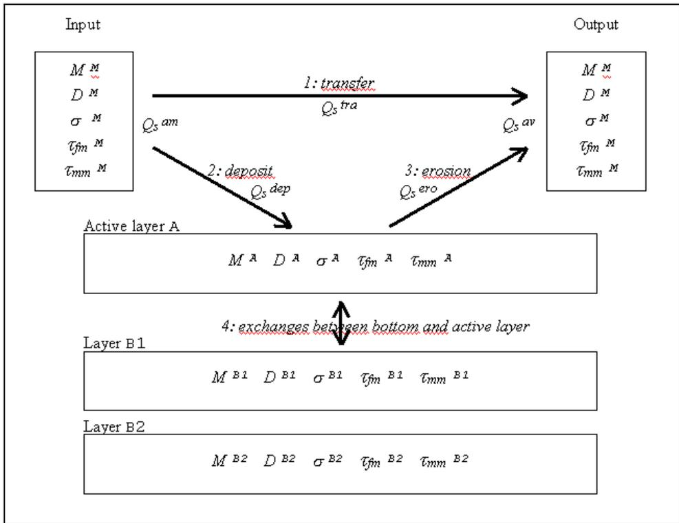
**Figure 2** Scheme of distribution of sediments inside one cell (Balayn, 2001)
