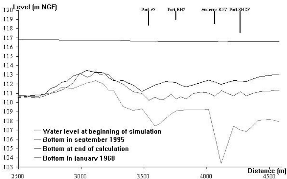
Figure 5 Comparison of the deposition process during the period 1968-1995 (Balayn, 2001)
