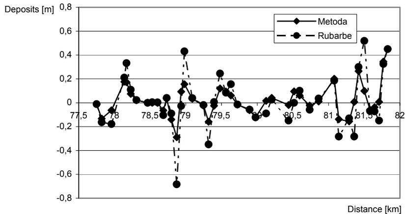
Figure 8. Bottom level change for steady flow  $Q = 250 \text{ m}^3/\text{s}$
