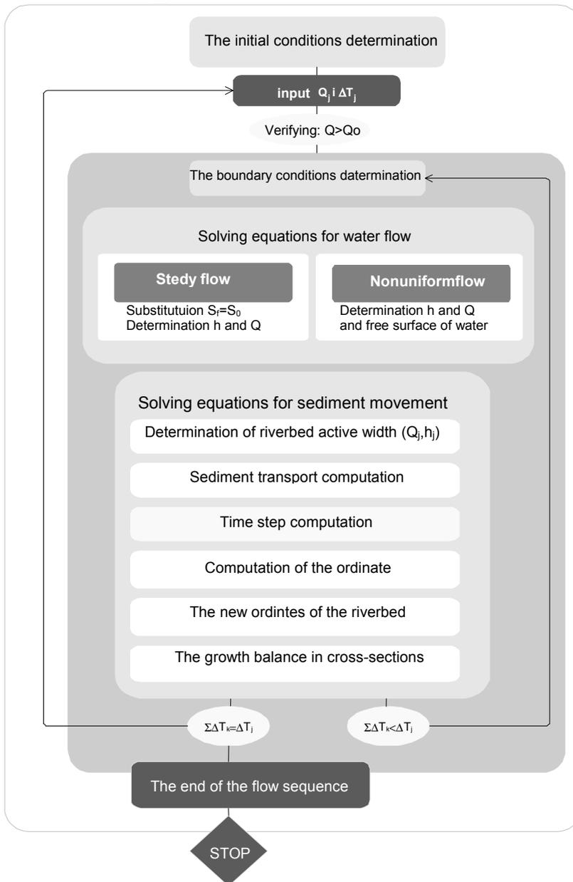
**Fig. 5 The block diagram of the METODA model.**
