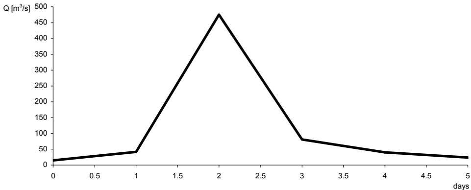
**Fig. 7 Flood discharge hydrograph.**
