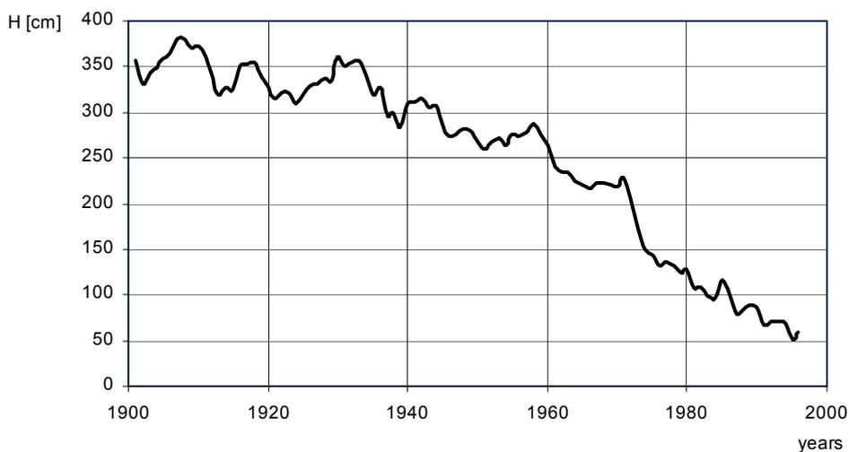
**Fig. 1 The riverbed erosion intensity on the experimental reach of the Raba River.**
