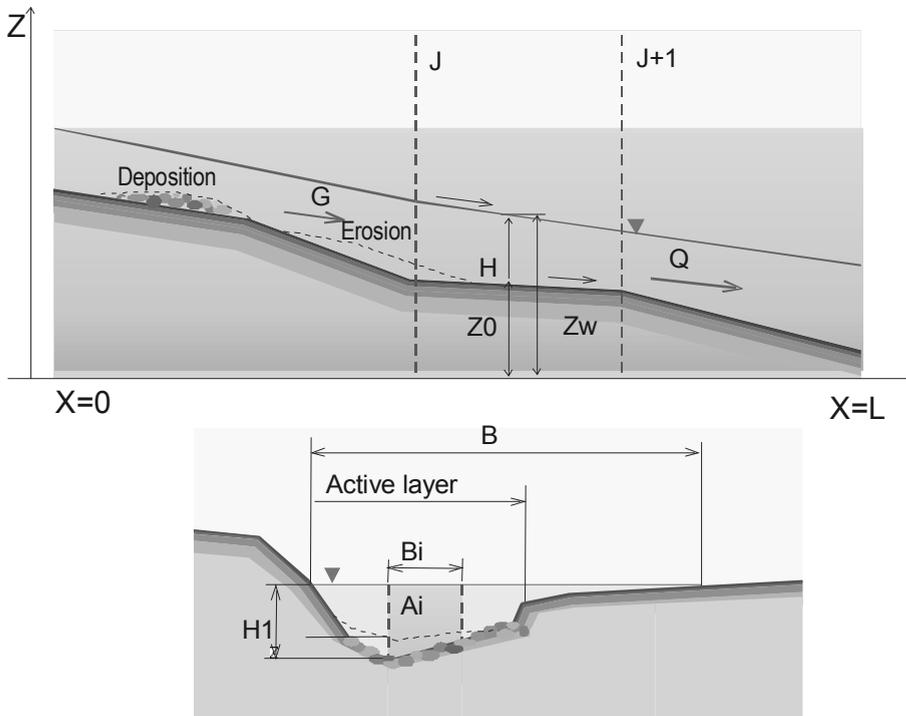
**Fig.4 The schematisation of longitudinal profile and cross-sections**
