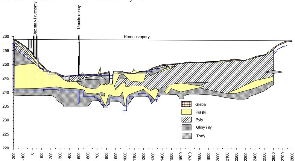
**Fig.3. Geological structure of the dam site with one aquifer**
