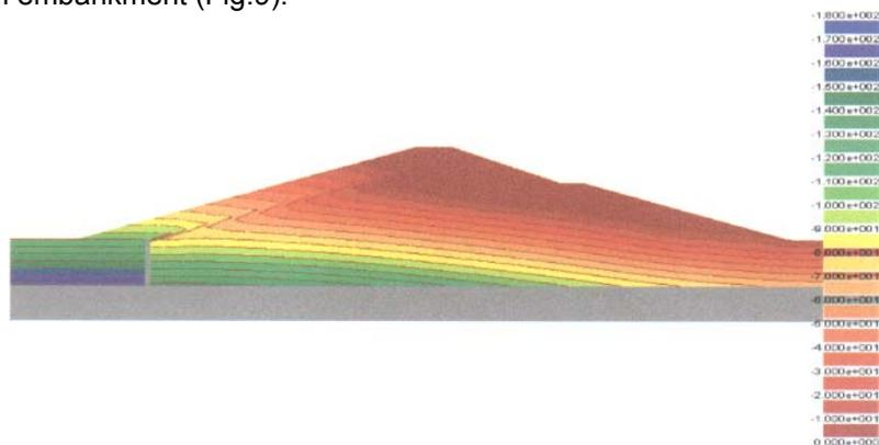
Fig.8. Simulation of the internal porewater pressure.
