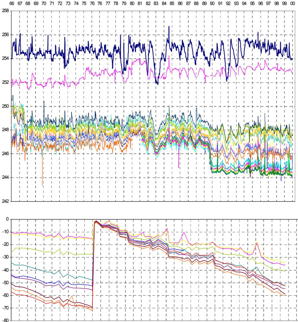
Fig.6 Reservoir level versus piezometric levels in years 1966 to 2001
