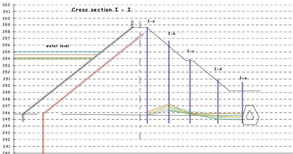
**Fig. 7. Piezometric level fluctuations in I cross-section**
