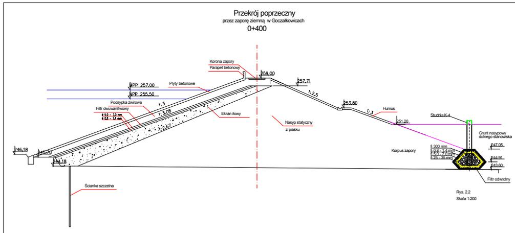
Fig. 5. Dam cross-section with clay screen
