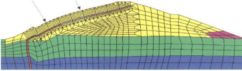
**Fig.9. Deformation of the embankment**
